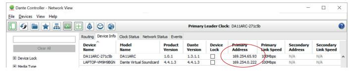
By accessing the IP address of the DA11ARC in your web browser, you will gain access the the units web GUI. The following details will allow you to log in to the admin section:
