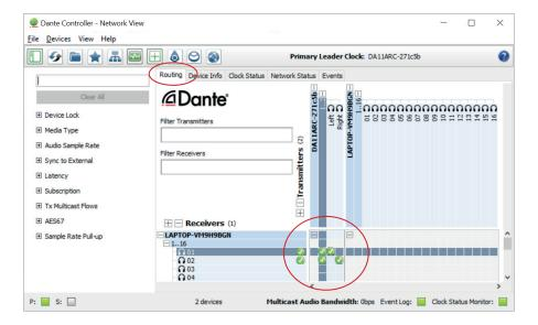
It is also possible to change the settings of the DA11ARC under the "Device Info" screen in the Dante Controller software. To do so, select the "Device Config" menu.
