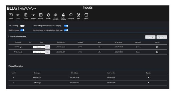
The top of the Inputs page lists all devices that are currently connected to the WMF51, as well as their connection type (dongles, Miracast, etc...). Renaming of dongles, and the ability to Operate the device (cast / stop) can also be managed from the top section of this page.
