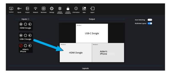
Available wireless connections are listed on the left hand side of the GUI. There are 3 action buttons for each connected device that can be used within this page.
