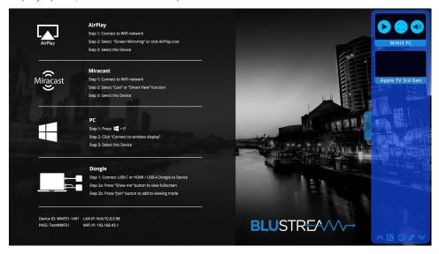
Wirelessly connected devices paired with the WMF51 can be seen as thumbnail views (please note: screen-grab thumbnails are not available for some wireless connections (i.e. Airplay)). The user can select any connected device to be displayed on the panel from this menu. Multiview, full screen and audio options can be managed from the icons overlayed on each thumbnail.
