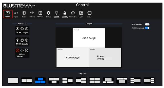
To switch the input device position to a different window of the multiview layout is as simple as dragging and dropping the left hand Input window onto the portion of the output graphic. Where (in the below example), the USB-C Dongle is dropped onto the HDMI Dongle window, the USB-C Dongle will be moved to the position where the HDMI Dongle was originally displayed, effectively swithcing their positions around:
