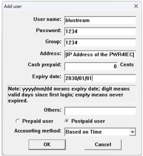
Use the IP address of the PWR8IEC in the address field. Click confirm to add the account
