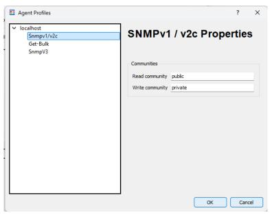
4. Navigate to Options/Manage SNMPv3 USM Profiles... and fill in the fields to match was what set under SNMP V3 in the Web-GUI.
