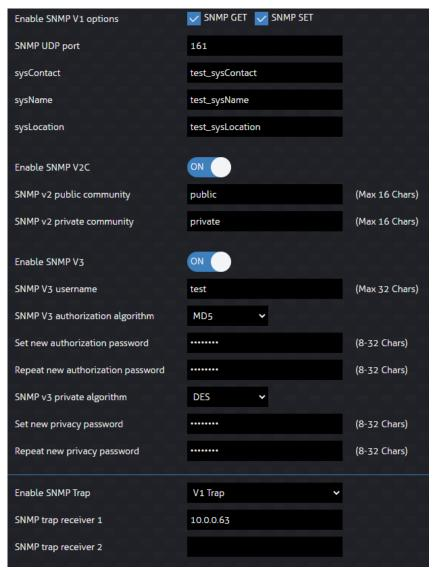
2. Open the snmpb software and navigate to Options/Manage Agent Profiles... and create a new user. Set the Agent Address to the IP address of the PWR8IEC and the port to the SNMP UDP port set in the Web-GUI.
