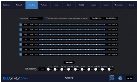
To adjust the logic for any given day, move the blue dots along the timeline to create a highlighted selection: this is when the device will power on. In order to add additional logic (i.e multiple on and off periods), press the + More Schedule button. You can now add additional logic by repeating the steps above.
